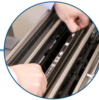
Quick Change Creasing Matrix Easy to swap in just seconds, with no tools required
