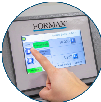
Touchscreen Control Panel Program jobs, switch between inches/mm, paper eject function, programming via cutting & more
