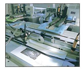
Kirk-Rudy's envelope flap opening section utilizes a pinch roller/plow assembly combined with a compressed air blast to positively open every flap. In the event a partially sealed flap is not opened, a flap detection circuit will automatically stop the machine.
