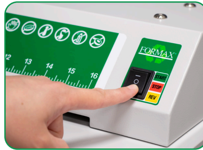
Simple Push-Button Control Start, stop, and reverse easily with a single toggle switch
